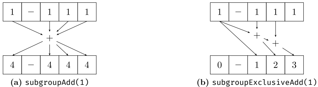
Figure 19: Subgroup operations on a subgroup of 4 active invocations and one inactive invocation. Inactive invocations contribute the value 0.
